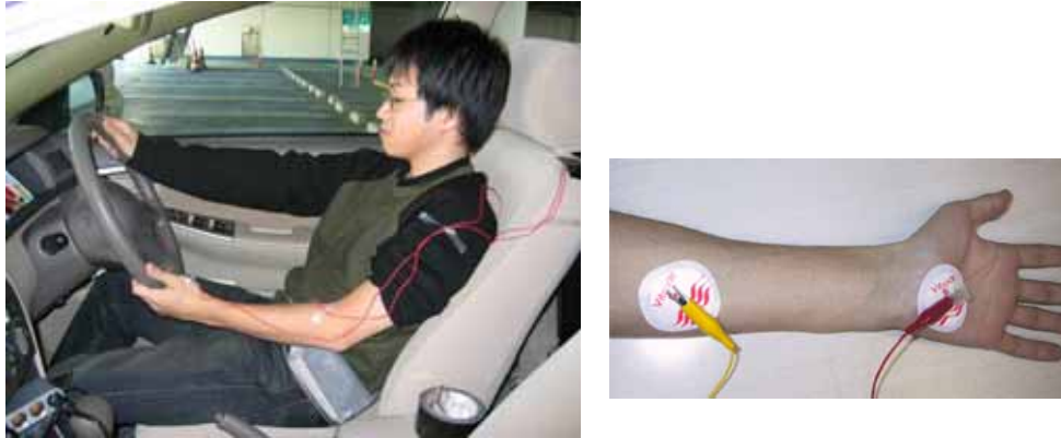
Figure 6-8 Skin potential level measuring
