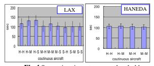
**Fig.4** Separation time at runway threshold (Los Angeles International Airport and Haneda)
